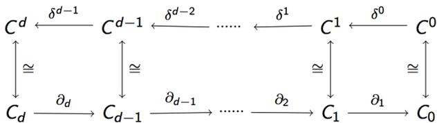
**Fig. 1.** Chain and cochain complex as a sequence of linear spaces of chains ( $C_d$ ), i.e. domain subsets, and cochains ( $C^d$ ), i.e. discrete fields, with linear boundary ( $\partial$ ) and coboundary ( $\delta$ ) operators, under constraints  $\partial_{d-1} \circ \partial_d = \delta_d \circ \delta_{d-1} = 0$ .
