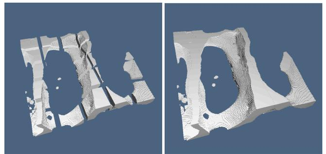
**Fig. 2.** Since the bottleneck of GPGPU is moving data from global to local memory, the extraction of model portions is done in parallel using the *same*  $[\partial_3]$  matrix for a  $n^3$  subimage.
