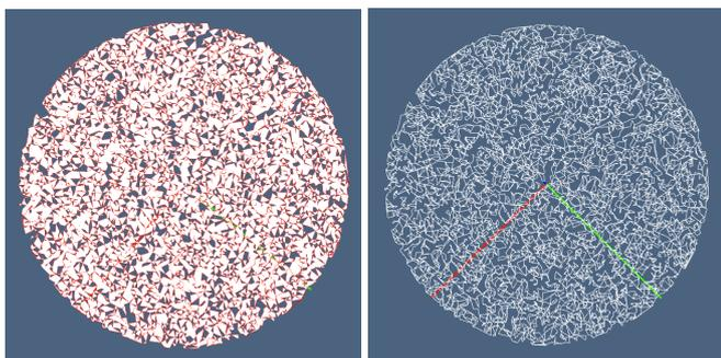
**Fig. 3.** (a) A random polygon in the unit circle; (b) the boundary of the total chain, computed by a single SpMV multiplication. The same  $[\partial_2]$  matrix is used to extract the boundary of *any* polygon subset.
